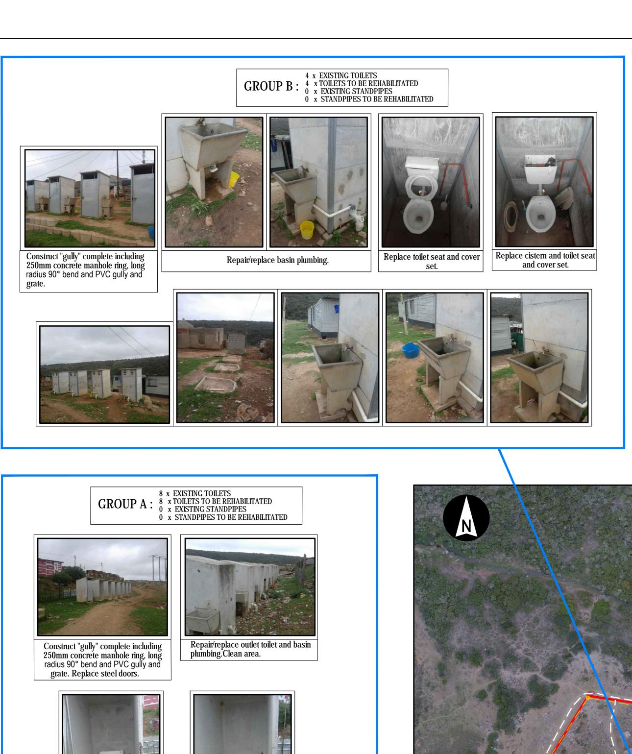
Replace cistem, poly cop pipes with fittings and connectors and toilet plumbing. Replace toilet seat and cover set.
